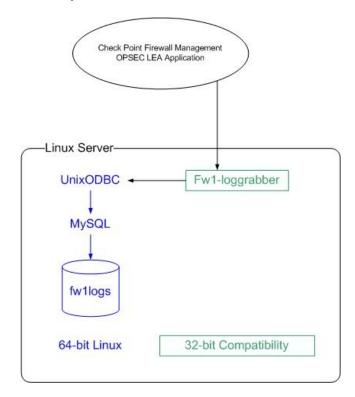
The fw1-loggrabber application on the database server pulls the Check Point log transactions via an SSL connection, then passes the data through UnixODBC to MySQL which stores it in the database.
